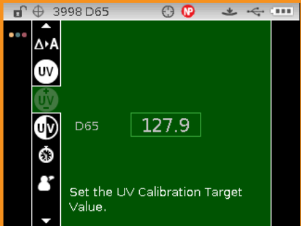
Calibrated UV component – first X-Rite handheld spectrophotometer with adjustable UV component to fully characterize optically brightened materials
