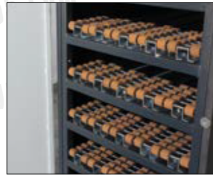
Top rollers carriage inside view.
