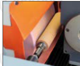
Long cots for Drawing and Combing Frames can be processed on the same machine without any complicated, time consuming conversions needed.
