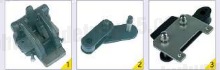
Mercerizing clip and chain Stenter brand: Japan Sando Machine
