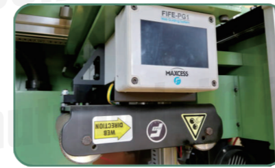
Imported deviation rectification system allows to have an accurate tracking
